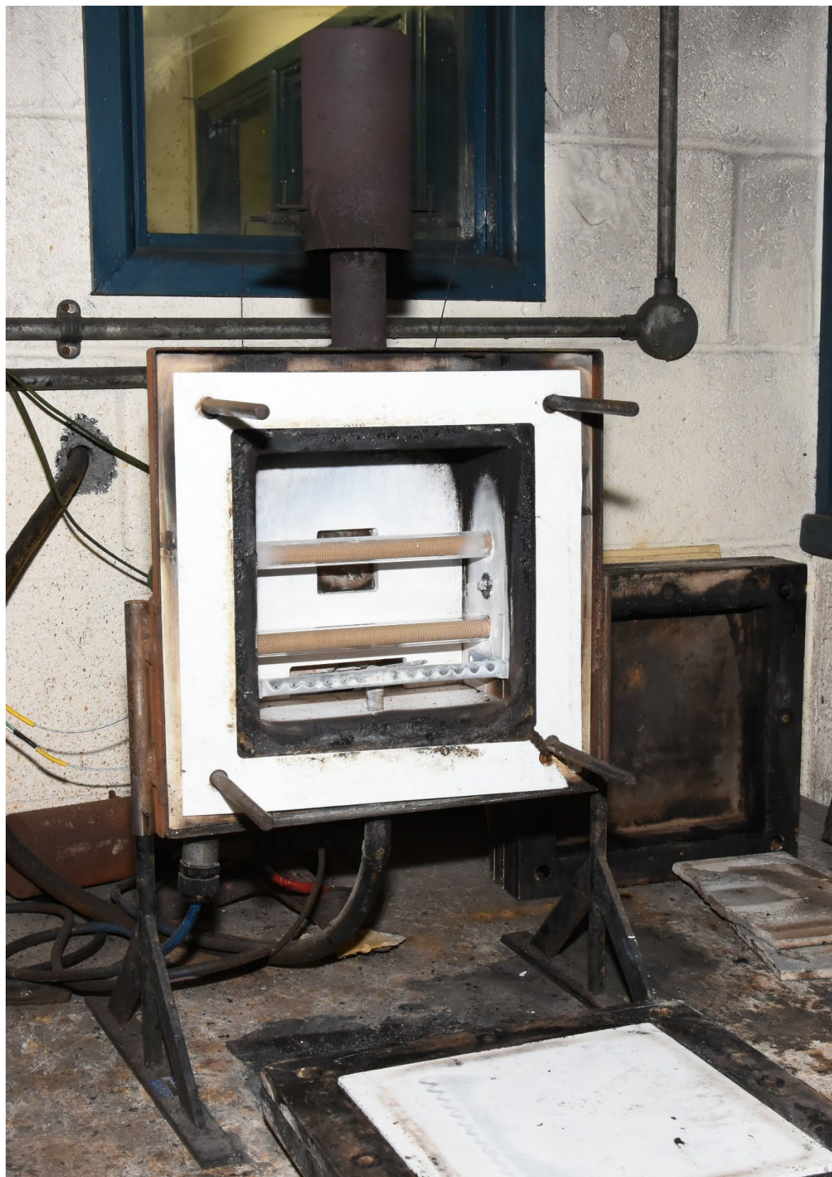
Figure A.3 – BS 476-6 test apparatus with specimen on bench in front of apparatus containing a blank specimen
