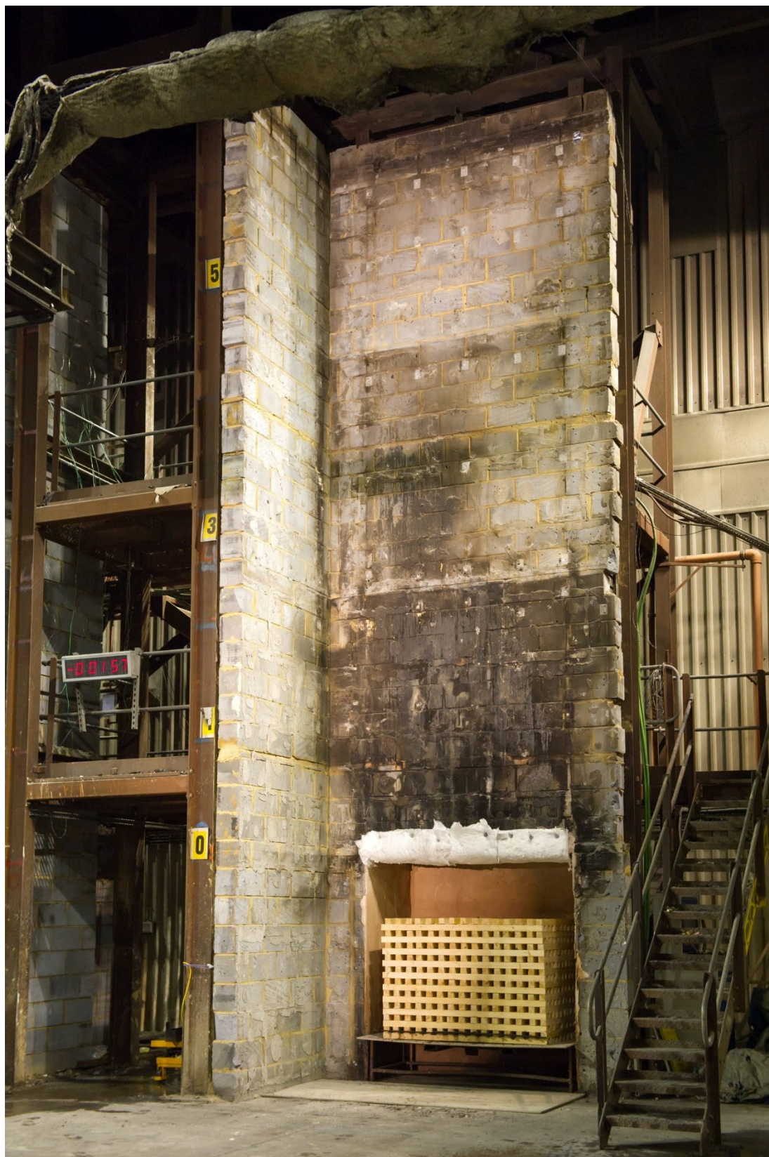
Figure A.9 – BS 8414-1 rig with a timber crib installed in the combustion chamber but no test specimen installed onto the rig
