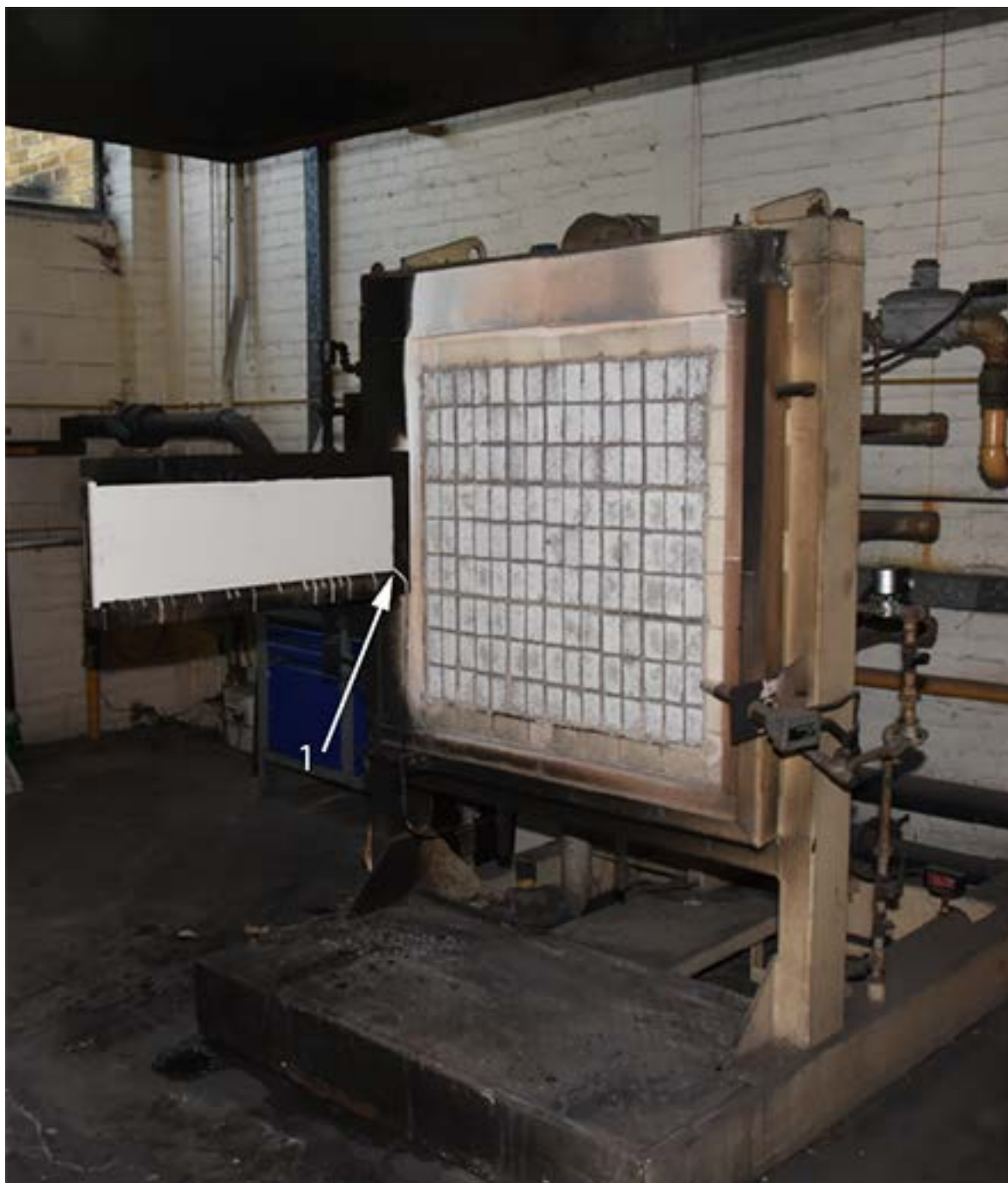
Figure L.1 – BS 476-7 test apparatus with specimen holder in position for test and containing a blank specimen
