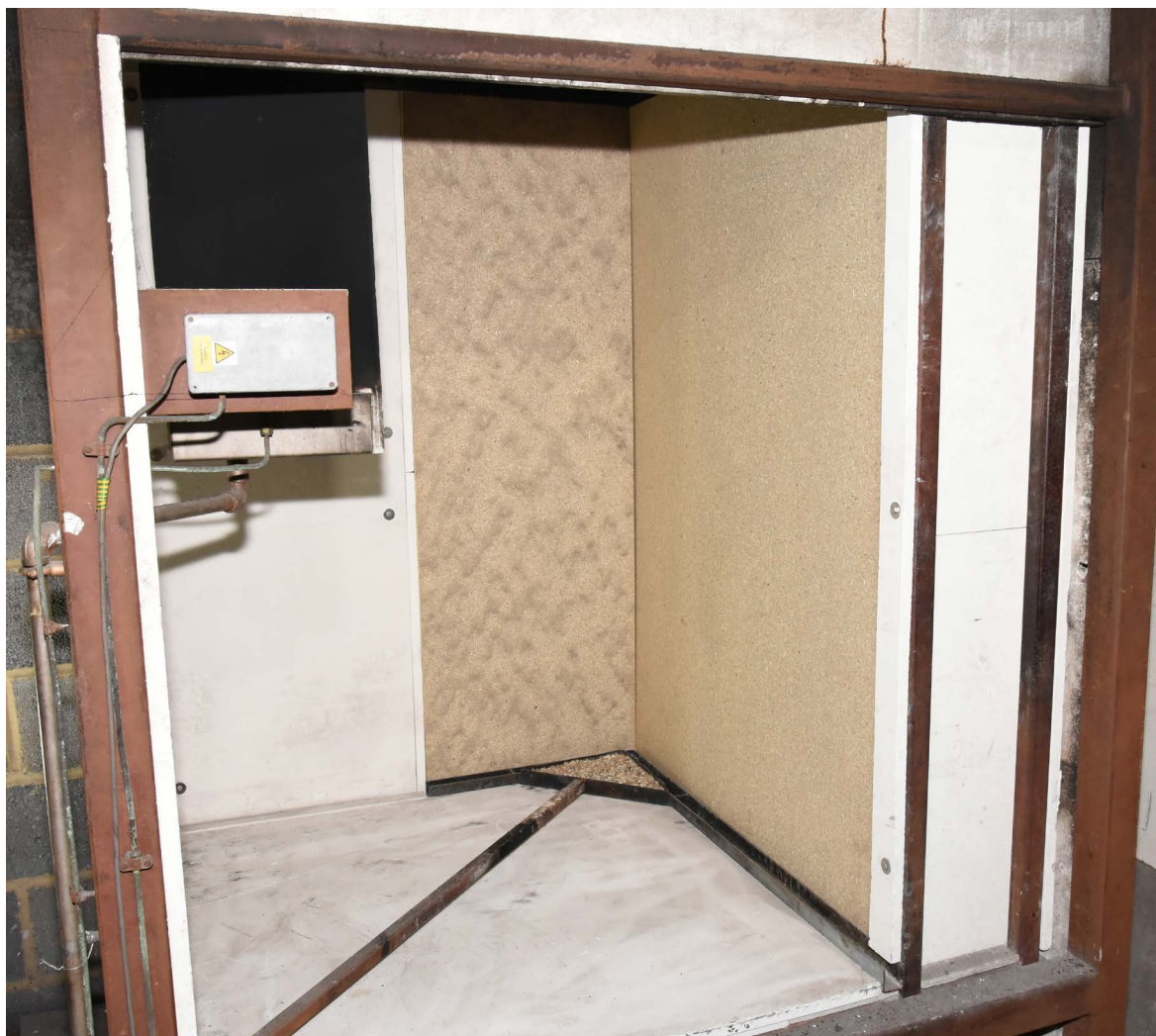
Figure L.5 – BS EN 13823 test apparatus with blank specimen in position for test
