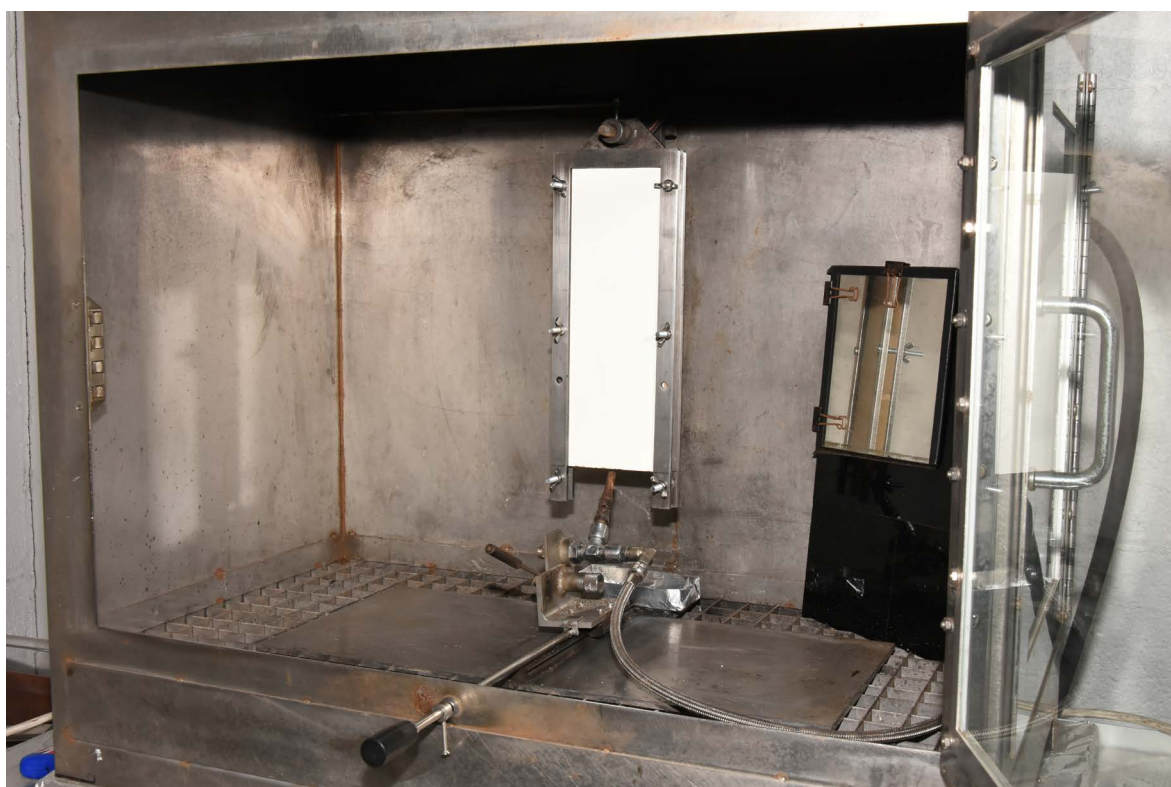
Figure L.4 – BS EN ISO 11925-2 test apparatus with blank specimen in position for test
