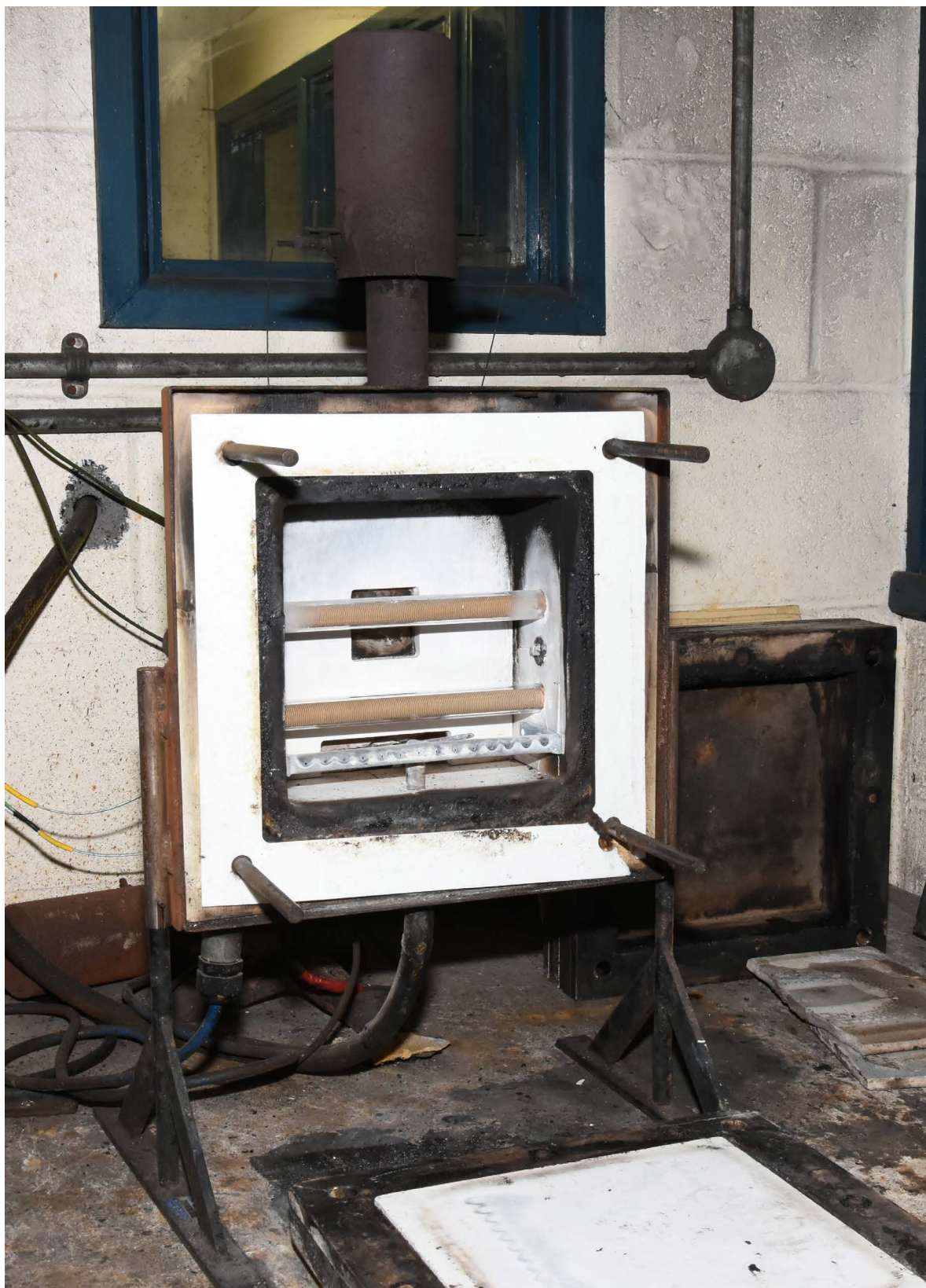
Figure L.3 – BS 476-6 test apparatus with specimen on bench in front of apparatus containing a blank specimen
